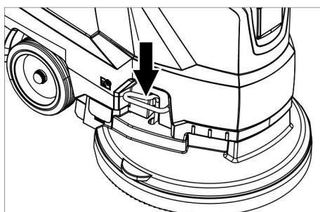
→ Pull the device towards the back so that the disc brush becomes accessible.
