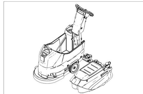
→ Lift up the waste water tank and put it aside.
