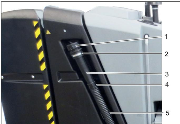
The waste water tank drain hose is located on the right-hand side of the device.
